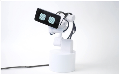
Figure 4: Robotic base with phone magnetically docked and charging
