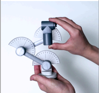
Figure 2: We prototyped animations with paper protractors stuck into the joints of a miniature 3D print we made of Baidu's AI robot by Teenage Engineering
